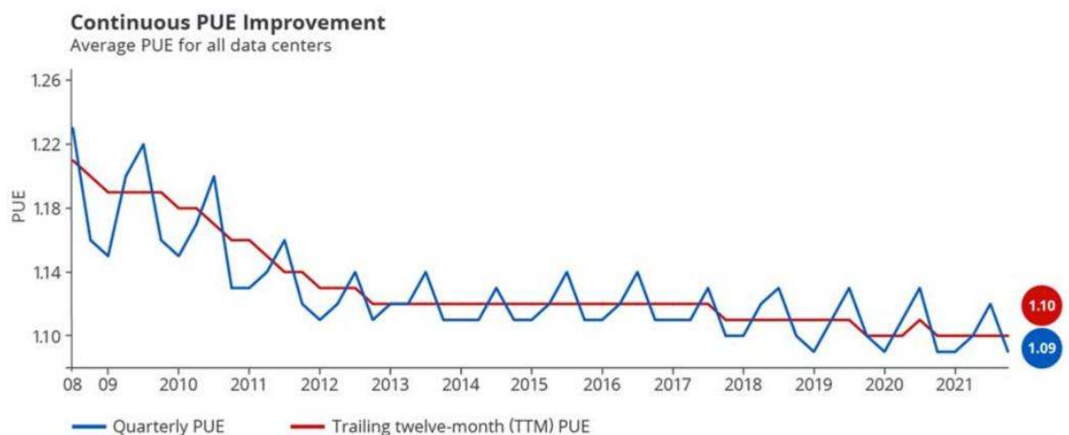
Figure 6.26 The PUE data for all Google WSCs, as reported at https://www.google.com/about/datacenters/efficiency/ .
