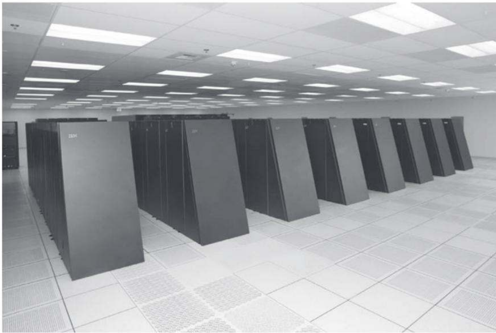
Figure I.19 The 64 K-processor Blue Gene/L system.
