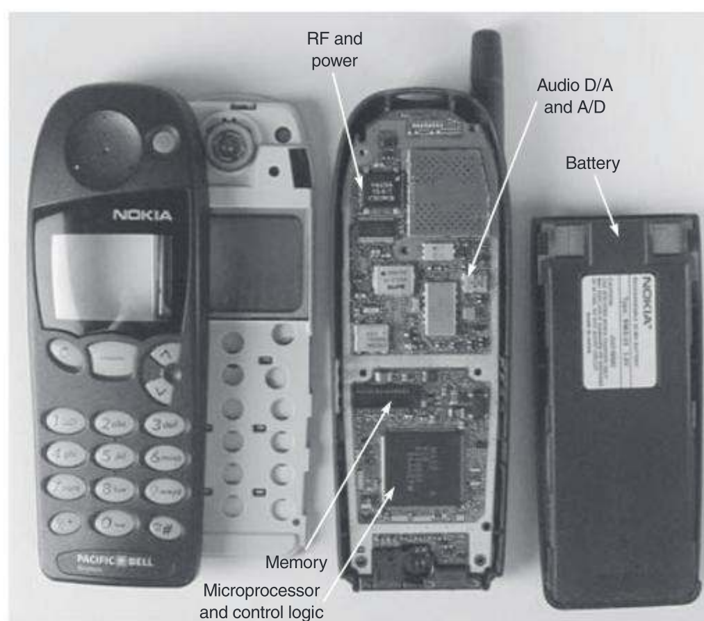
Figure E.17 Circuit board from a Nokia cell phone. (Courtesy HowStuffWorks, Inc.)
