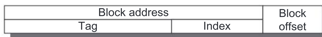
Figure B.3 The three portions of an address in a set associative or direct-mapped cache. The tag is used to check all the blocks in the set, and the index is used to select the set. The block offset is the address of the desired data within the block. Fully associative caches have no index field.
