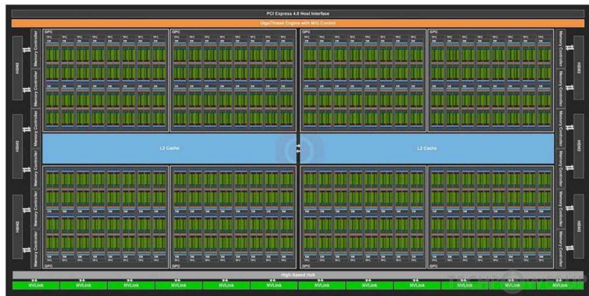
Figure 7.19 Floorplan of the NVIDIA A100. While it shows 128 SMPs, NVIDIA enables only 108 of them. The L2 cache holds 40 MB. The A100 can compress data from DRAM into the cache to accelerate unstructured sparsity and other compressible data patterns. The claim is that compression yields up to 4X of the DRAM read/write bandwidth, up to 4X of the L2 read bandwidth, and up to 2X of the L2 cache capacity.
