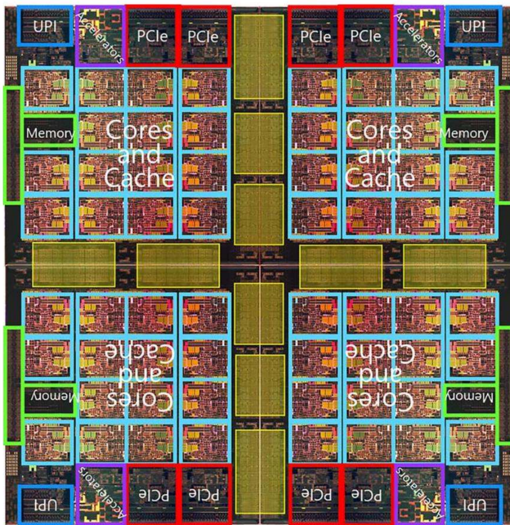
Figure 1.15 Microprocessor die components in Figure 1.14 are labeled with their functions. UPI (Ultra Path Interconnect) is an Intel point-to-point interconnect between sockets. PCIe (Peripheral Component Interconnect Express) is a standard, high-speed serial expansion bus to GPUs, network interfaces, and storage devices. The Memory block is the memory controller for DDR5 DRAM. The Accelerators block includes hardware support for the Advance Matrix Extension (AMX), the Advance Vector Extension (AVX), an engine to accelerate cryptography and data compression/decompressions (QuickAssist Technology), and the aptly named Data Streaming Accelerator (DSA). (There is also a version of Sapphire Rapids that is packaged with High Bandwidth Memory, and the HBM interface is also in the Accelerator block.)
